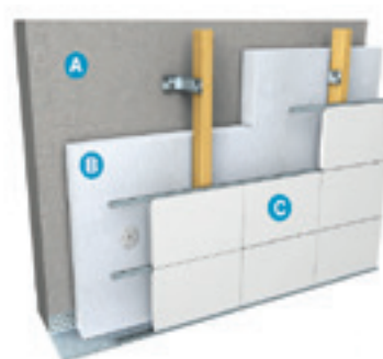
A Mur support B Panneau PSE Ther ULTRA Th C Bardage support
