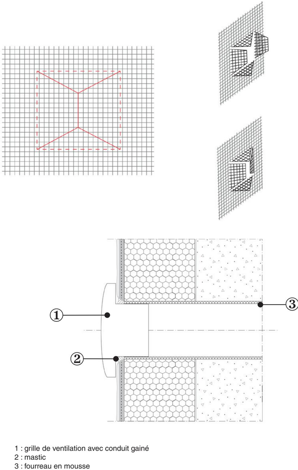
*Figure F1 – Orifice de ventilation*
